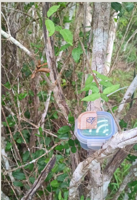
An Audiomoth (acoustics device) deployed in the reserve to record owl calls
